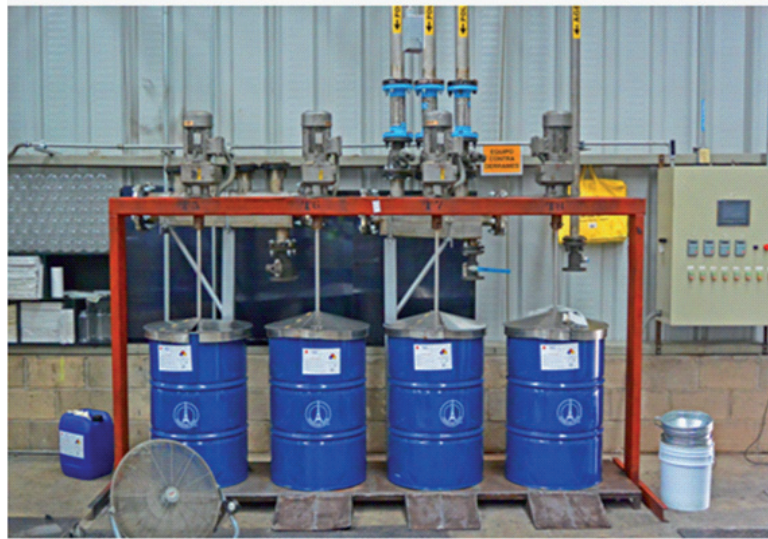
Example of a system house blending system
